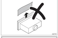
Do not remove the protective film between the deflector plate and the casing until the hood has been placed in the housing unit.
